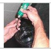
Lubricate new o-ring with supplied lubricant.
