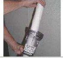
Place new cartridge into sump and tighten sump with sump wrench to a snug fit.
